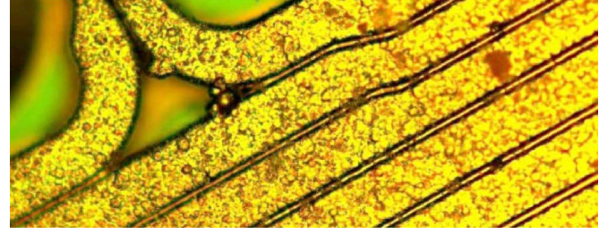
Fig. 3. Optical microscope photo of the plated magnetic layer on the outer frame. NiFe is deposited on existing Au coil windings for convenience (coil structure is not needed).
